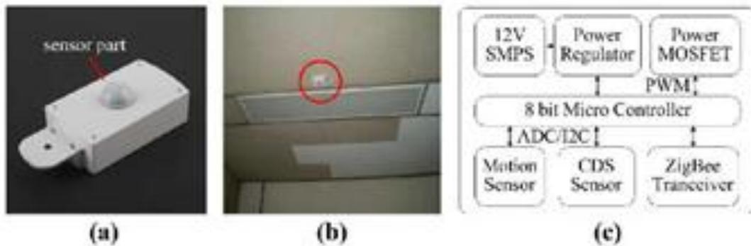
Fig. 4. Implementation of the proposed system; (a) prototype, (b) installation, (c) hardware block di
