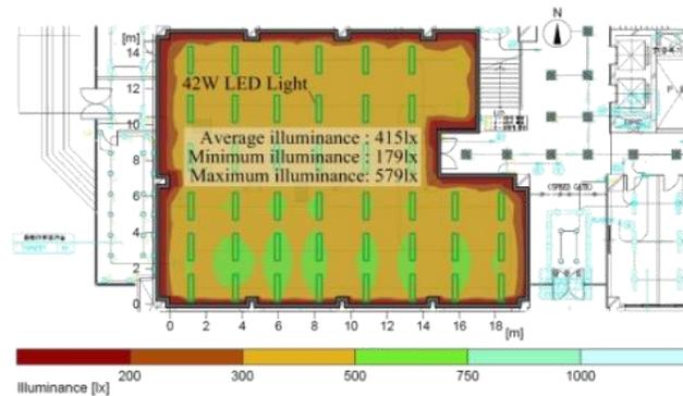
Fig. 5. Floor plan of a test bed with the illumination simulation result
