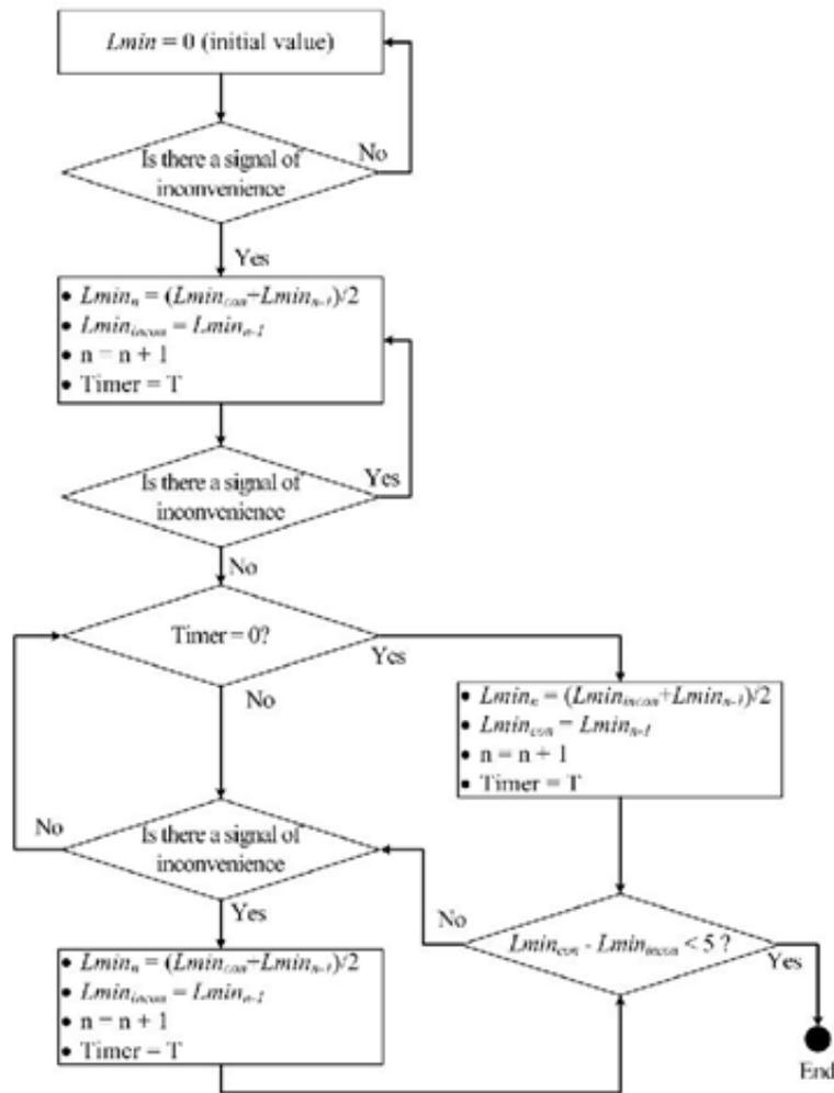
Fig. 3. flowchart of a minimum light intensity control algorithm
