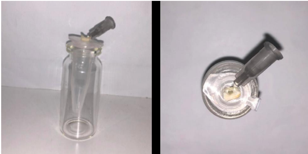
Fig. 1:- Experimental system used to evaluate the debris extrusion.
