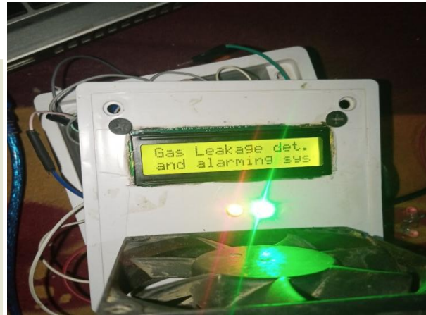
Figure 12:- Implementation and simulation results showing Gas leakage/smoke Detected and Red LED Light and Alarming system ON.
