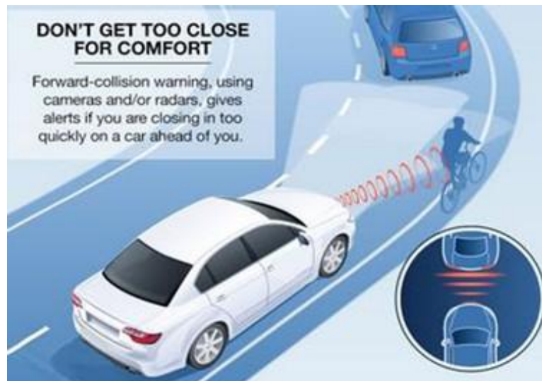
Fig. 1:- Schematic of a 77 GHz automotive radar system for VRU detection showing signal reflections from cyclists.
